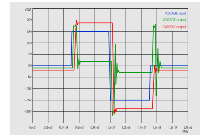
Fig. 2: iTRON AA current amplifier simulation
