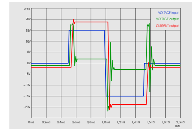
Fig. 2: iTRON AA current amplifier simulation
