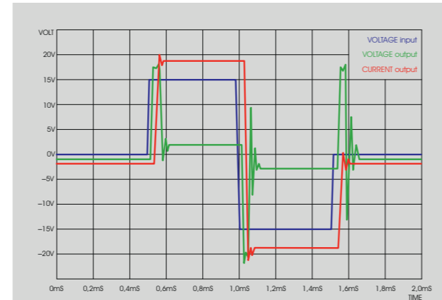
Fig.. 2: iTRON AA current amplifier simulation
