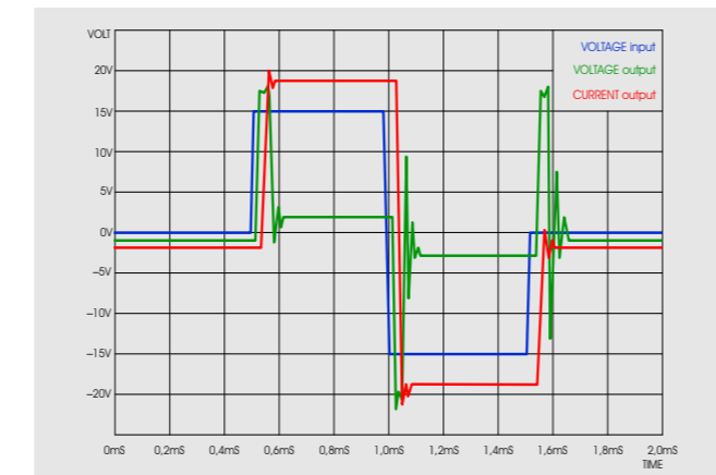
Fig. 2: iTRON AA current amplifier simulation
