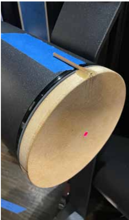
Axis alignment disc attached to the front of a trio tweeter module.
