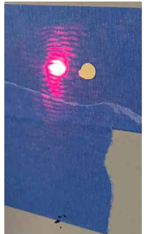
...and the spot /target marked on tape at the listening position. Careful adjustment and spot and target coincide exactly.
